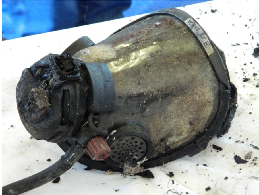
***Lt. Wallace's SCBA face mask with regulator melted. Thermal damage was attributed to flashover exposure and was secondary to running out of air.
