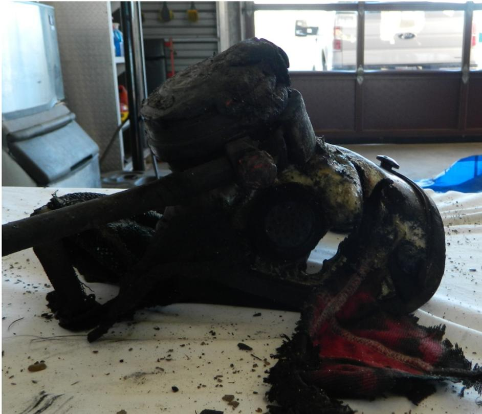
***Lt. Pickard's SCBA face mask with a hole melted through the lens. The mask was compromised and may have allowed for the inhalation of super-heated gases.
