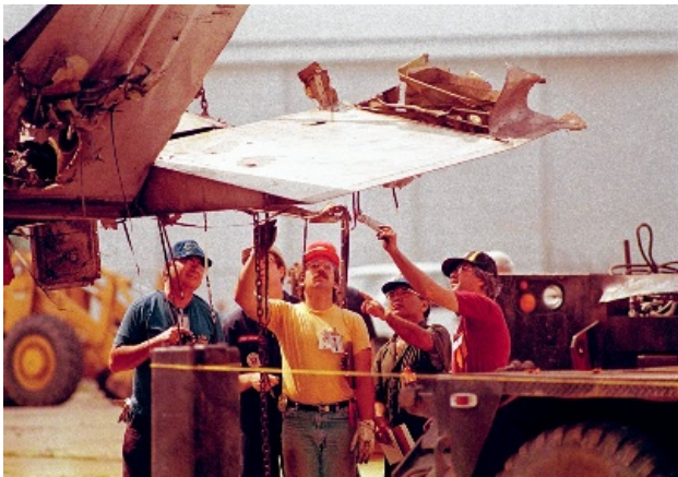
Jeff Davis, Associated Press file Inspectors look at the torn right horizontal stabilizer of Flight 232 on July 24, 1989.
