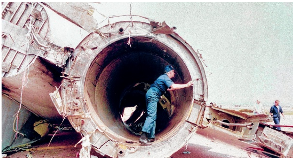
Ed Porter, Sioux City Journal file ABOVE: A National Transportation Safety Board inspector looks at the rear engine mount of Flight 232 on July 21, 1989.
