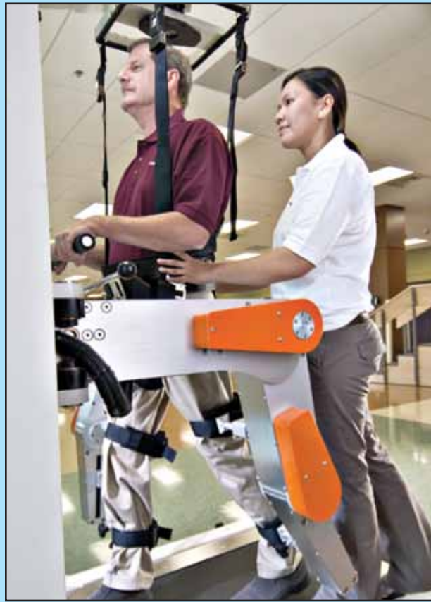
AutoAmbulator®, a sophisticated treadmill, allows body weight-supported ambulation and robotics to help patients with gait disorders.
