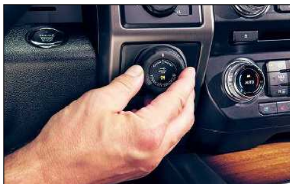
A new feature in the F-150 lets you steer a trailer by turning a knob left or right.
