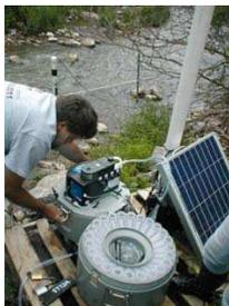
Fig. 4a. Servicing “R<sub>2</sub>D<sub>2</sub>” the Teledyne ISCO automated water sampler located at the Rt 38A site. It collected 1-liter of water daily (4 am) and was serviced bi-monthly.
